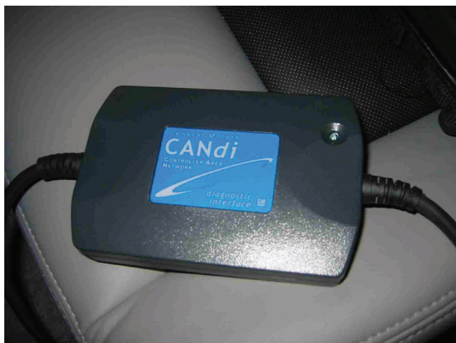
FIGURE 12 A CANDi module will flash the green LED rapidly if communication is detected.
