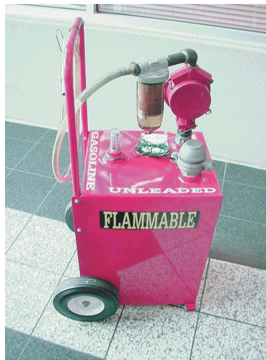
FIGURE 8 This red gasoline container holds about 30 gallons of gasoline and is used to fill vehicles used for training.
