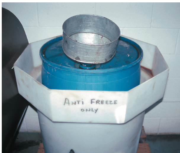
FIGURE 7 Used antifreeze coolant should be kept separate and stored in a leakproof container until it can be recycled or disposed of according to federal, state, and local laws. Note that the storage barrel is placed inside another container to catch any coolant that may spill out of the inside barrel.
