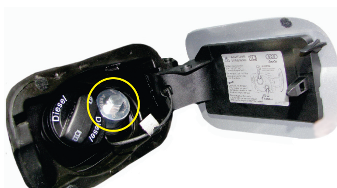
FIGURE 50 DEF is added to many light-duty vehicles through a fitting located near the fuel filler door.
