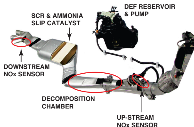
FIGURE 49 The upstream and downstream NOx sensors provide data for OBD-II aftertreatment system monitoring and not closed-loop feedback of metered DEF fluid. Incorrect type of DEF fluid and DEF dosing problems are also diagnosed by the sensors.
