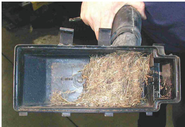
FIGURE 4 Any fault in the air cleaner assembly can disrupt the airflow through the MAF sensor.
