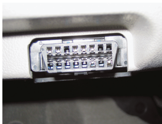
FIGURE 16 A typical OBD-II data link connector (DLC). The location varies with make and model and may even be covered, but a tool is not needed to gain access. Check service information for the exact location if needed.
